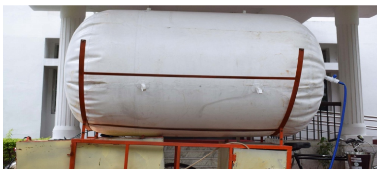
Figure: Balloon used to fill biogas and transport at various locations through chai-thela rickshaw
